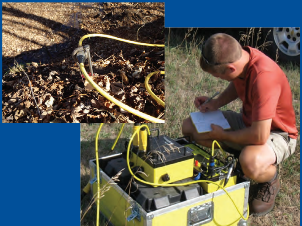
FIGURE 2. Collecting electrical resistivity field data. Meter, switch box, batteries (main photo), cables, and electrodes (upper left).
